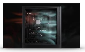
XPG VALOR AIR sports a sleek, clean look with a streamlined design that enhances cool air from outside to be drawn in via x3 pre-installed 120mm fans at the front, and a 120mm fan at the rear to exhaust the heat.
