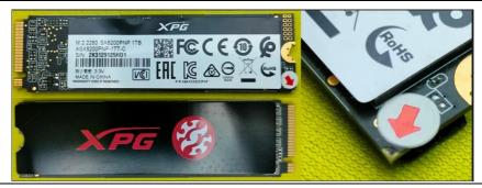
Screw hole has broke or oxidised
