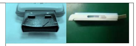
Damaged and scratched on the connector or/and SN number and capacity are unrecognized.
